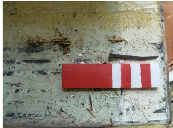
19 th century nail from dismantled side closed string section removed when plywood removed [10cm Scale]
