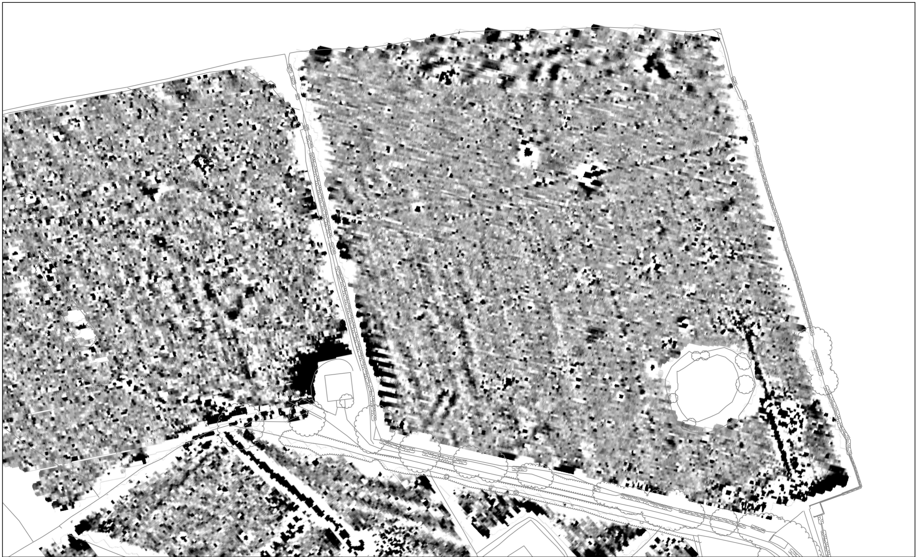
MSSD09 - Proposed Development at Brook Farm, Dowbridge, Kirkham Figure 7 - Magnetic Survey - Greyscale Plot - Area 3 1 : 1,000 @ A3
