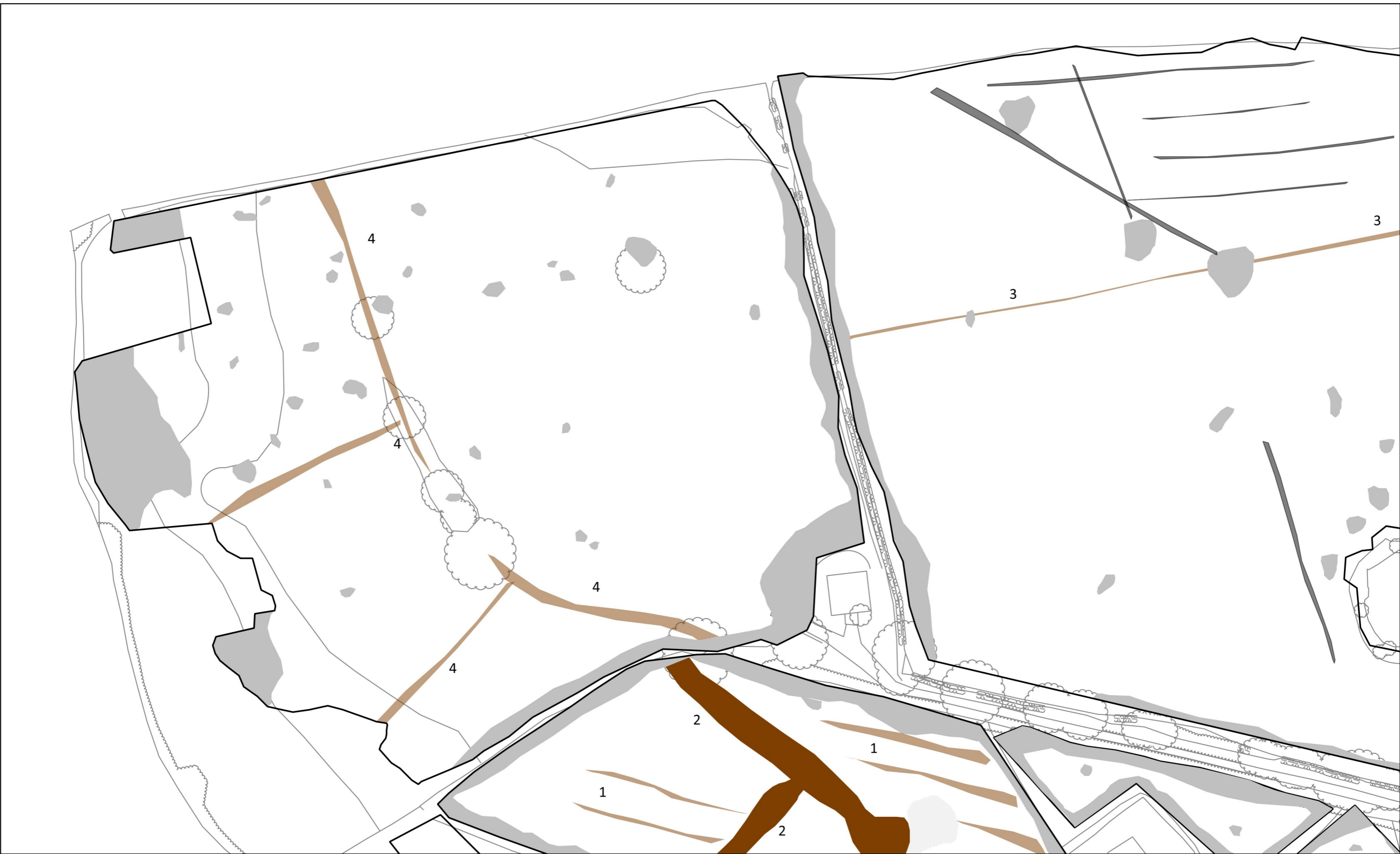
MSSD09 - Proposed Development at Brook Farm, Dowbridge, Kirkham Figure 6 - Magnetic Survey - Interpretation - Area 5 1 : 1,000 @ A3
