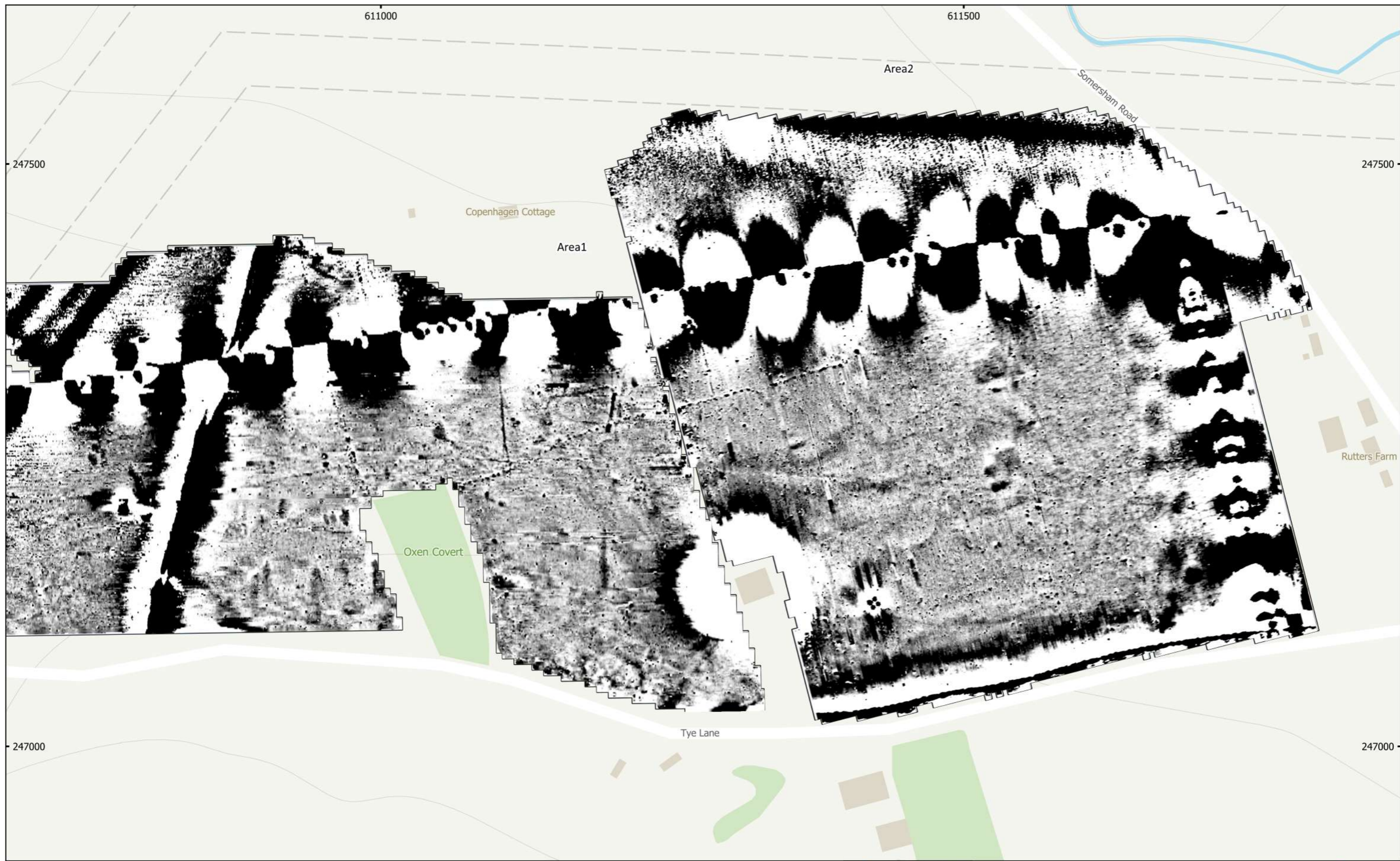
MSTM817 - Tye Lane Solar Farm Figure 5 - Magnetic Total Field (Lower Sensor) (Overview) (East Overview) 1:1,3000 @ A3 Copyright Magnitude Surveys Ltd 2022 Contains Ordnance Survey data © Crown Copyright and database right 2022
