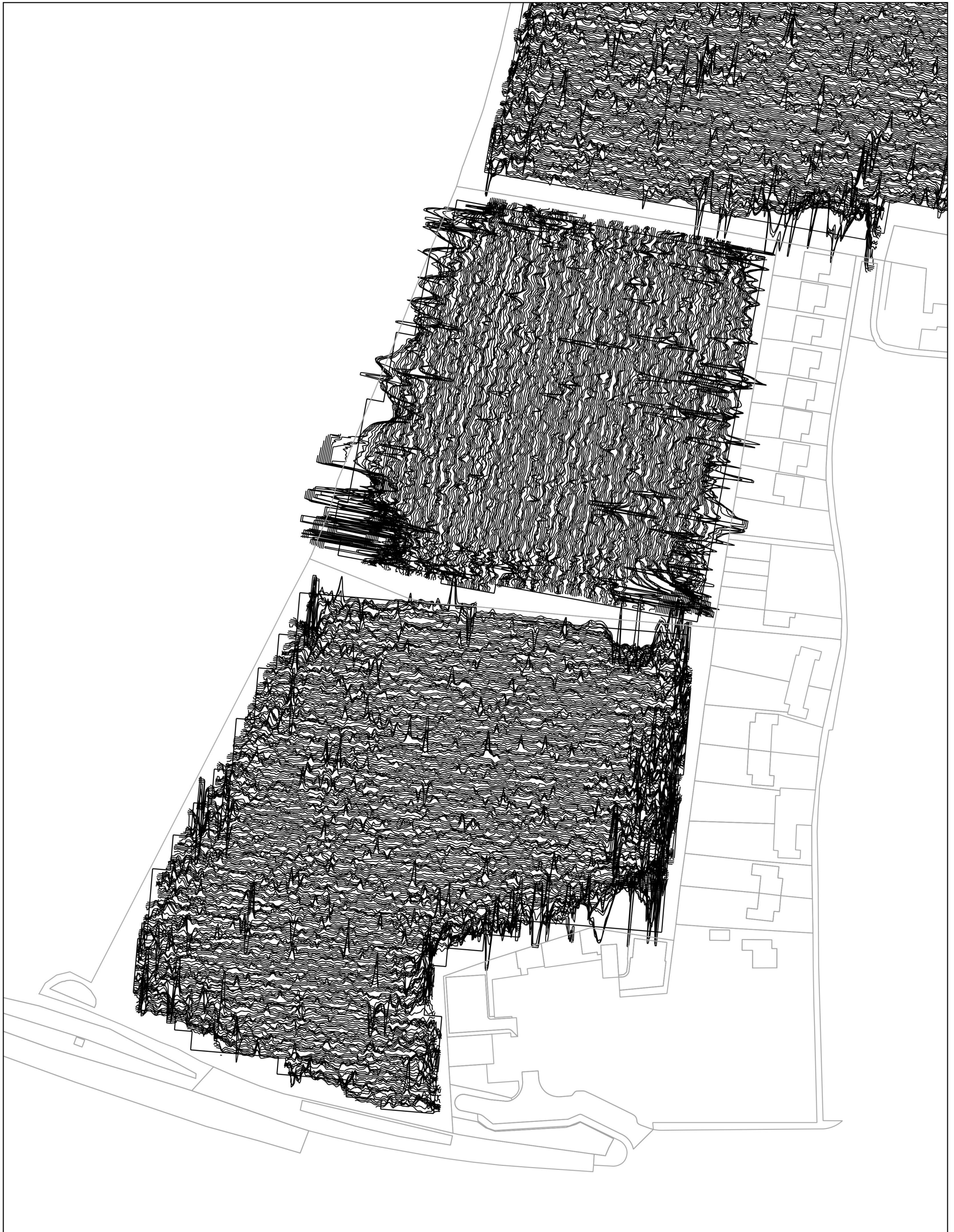
MSSK17 - Geophysical Survey at Heather, Leicestershire Figure 9 - Magnetic XY Trace 1 : 1000 @ A3 Copyright Magnitude Surveys Ltd 2016 Contains Ordnance Survey data © Crown Copyright and database right 2016 OS (100056946) XY Trace 15nT per cm @ 1:1000
