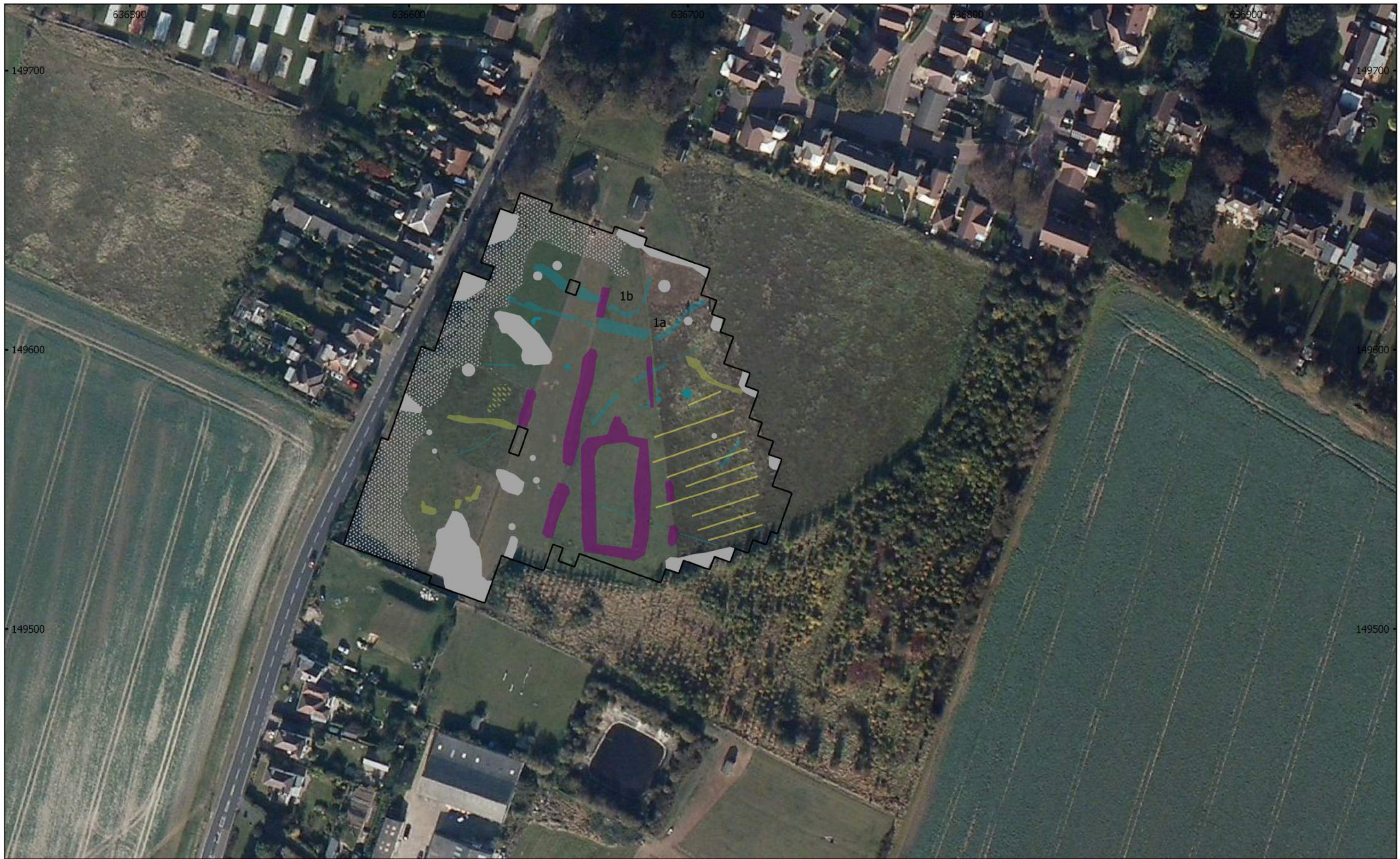
MSTR117 - Land at Dover Road, Deal, Kent Figure 5 - Magnetic Interpretation Over Satellite Imagery 1:1250 @ A3 Copyright Magnitude Surveys Ltd 2017 Contains satellite imagery: © 2017 Bing
