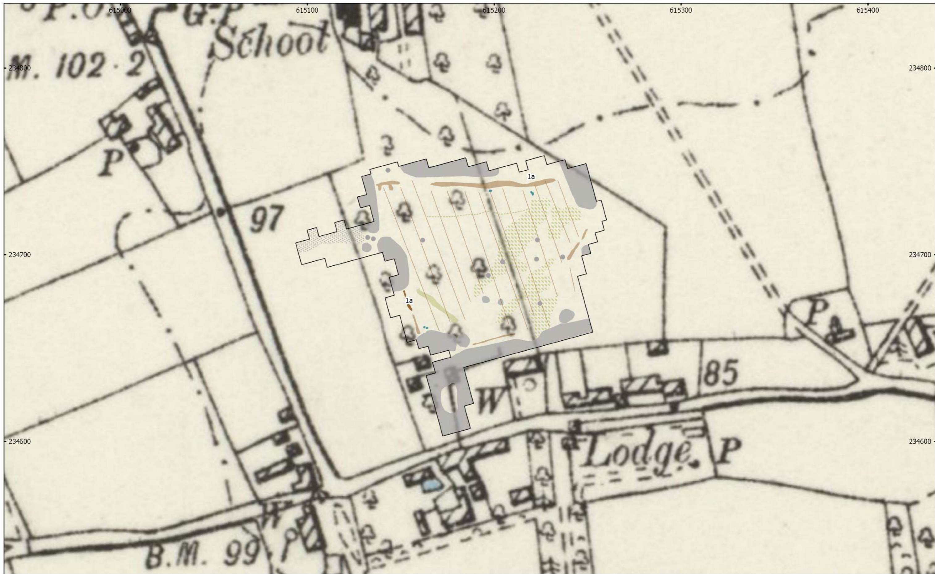
MSTM388 - Land at Church Road, Stutton Figure 7 - Magnetic Interpretation Over Historic Maps 1:1,250 @ A3 Copyright Magnitude Surveys Ltd 2018 Contains historic maps: Ordnance Survey, 6" 2nd edition c. 1882-1913 © National Library of Scotland
