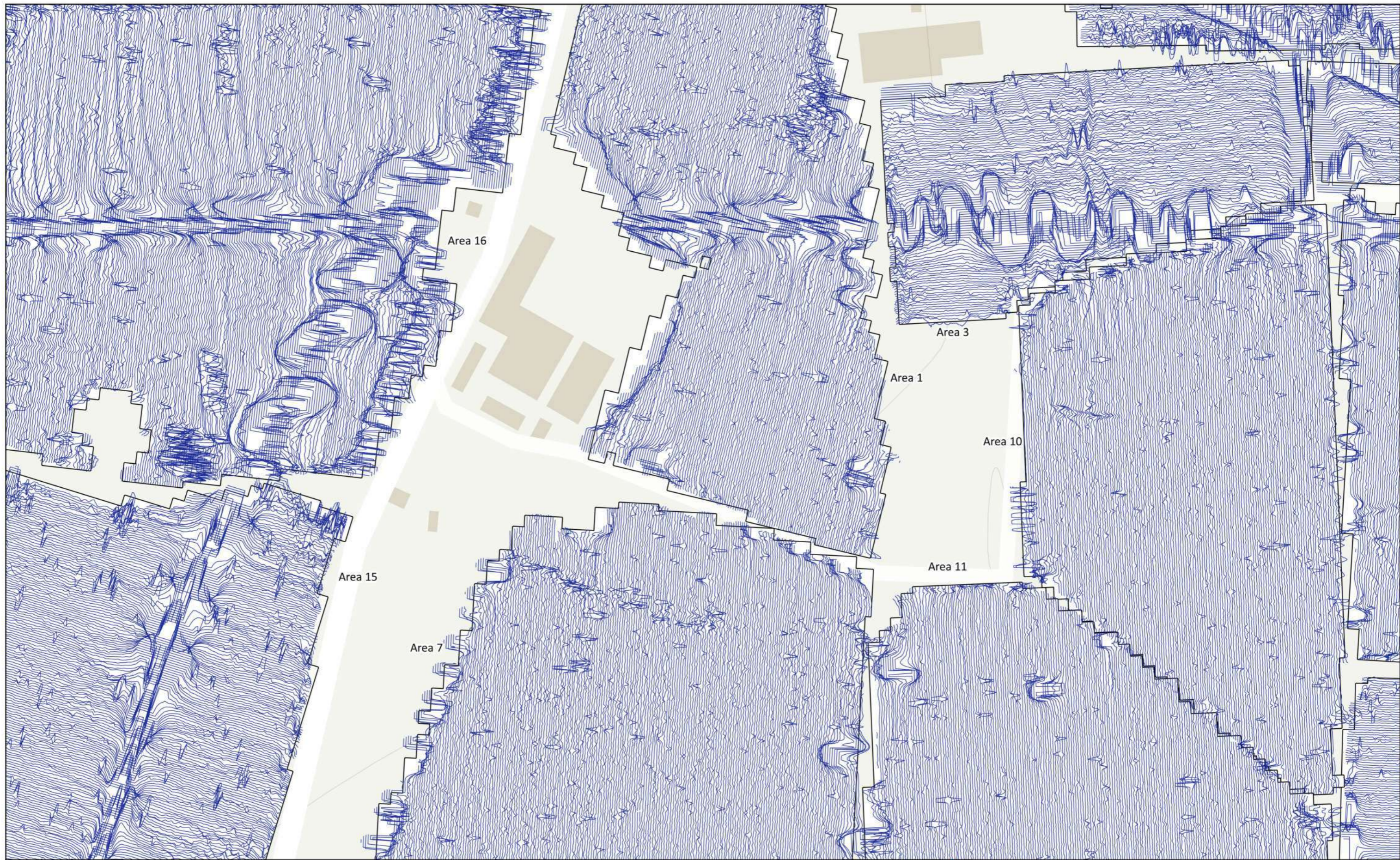
MSSO722 - Land to the East of A38 and North of A419, Whitminster, Stroud Figure 25 - XY Trace Plot (Areas 3, 10, 1, 11, 7, 15 & 16) 30nT/cm at 1:1,500 @ A3 Copyright Magnitude Surveys Ltd 2020 Contains Ordnance Survey data © Crown Copyright and database right 2020
