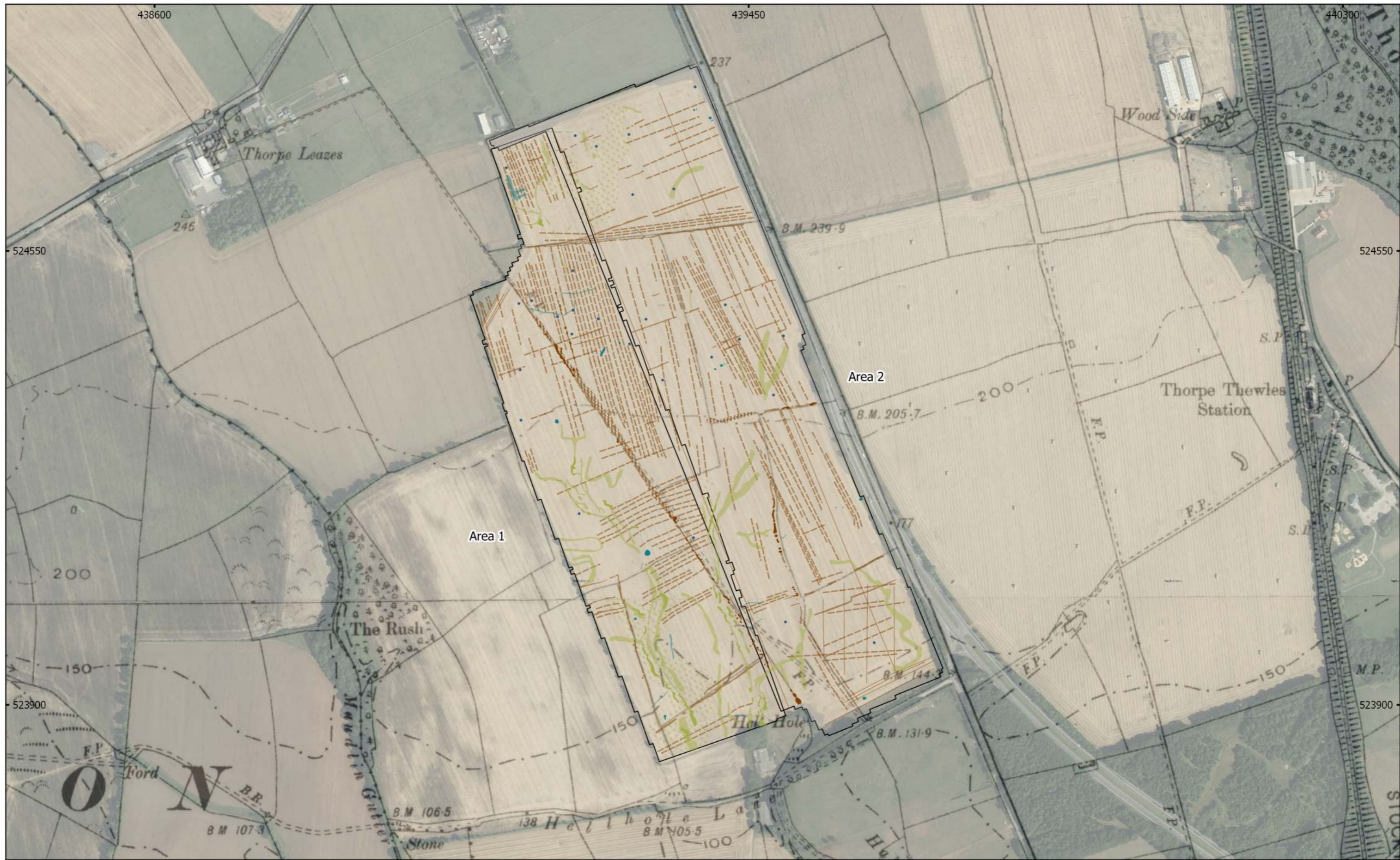
MSNZ728 - Thorpe Bank Solar Farm, Thorpe Thewles Figure 4 - Magnetic Interpretation Over Historic Maps and Satellite Imagery (Overview) 1:5,000 @ A3 Copyright Magnitude Surveys Ltd 2020 Contains satellite imagery © 2020 Bing Satellite Contains historic maps: Ordnance Survey, 6" 2nd edition c. 1882-1913 © National Library of Scotland
