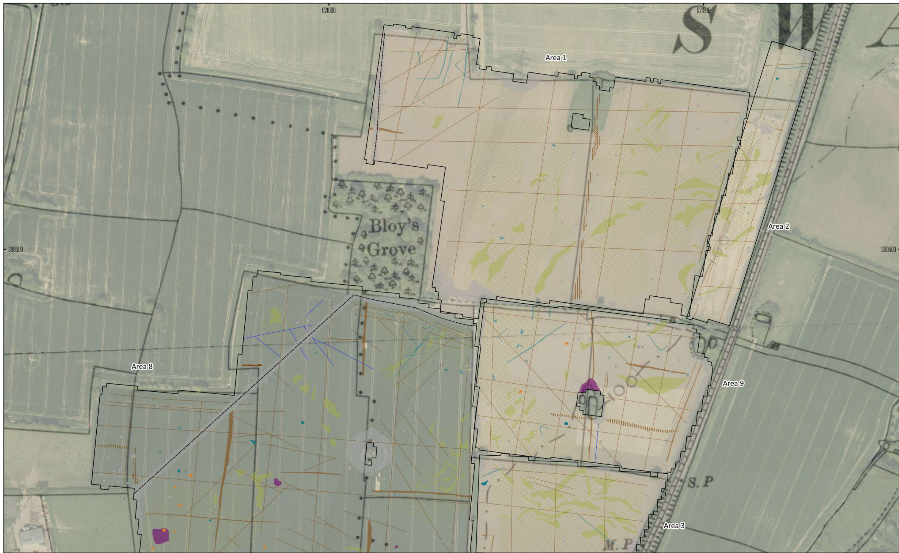
MSTM870 - Bloy's Grove Solar Farm, Swainsthorpe Figure 4 - Magnetic Interpretation Over Historical Maps and Satellite Imagery (Overview) (North) 1:3,000 @ A3 Copyright Magnitude Surveys Ltd 2021 Contains historic maps: Ordnance Survey, 6" 2nd editionc. 1882-1913. Reproduced with the permission of the National Library of Scotland. Contains Satellite Imagery © 2021 Bing Satellite
