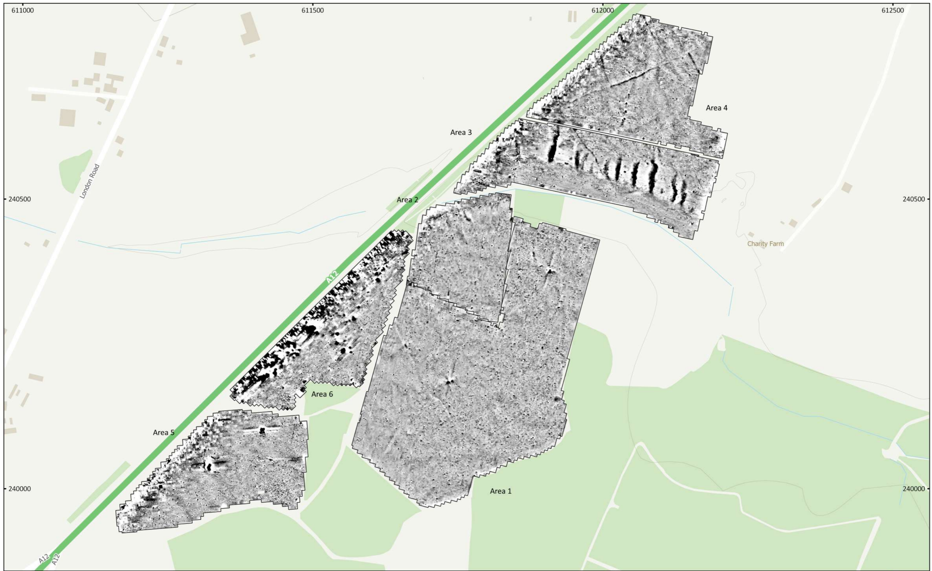
MSTM970 - Proposed Quarry, Brockley Wood, Belstead, Suffolk Figure 3 - Magnetic Total Field (Lower Sensor) (Overview) 1:4,000 @ A3 Copyright Magnitude Surveys Ltd 2021 Contains Ordnance Survey data © Crown Copyright and database right 2021
