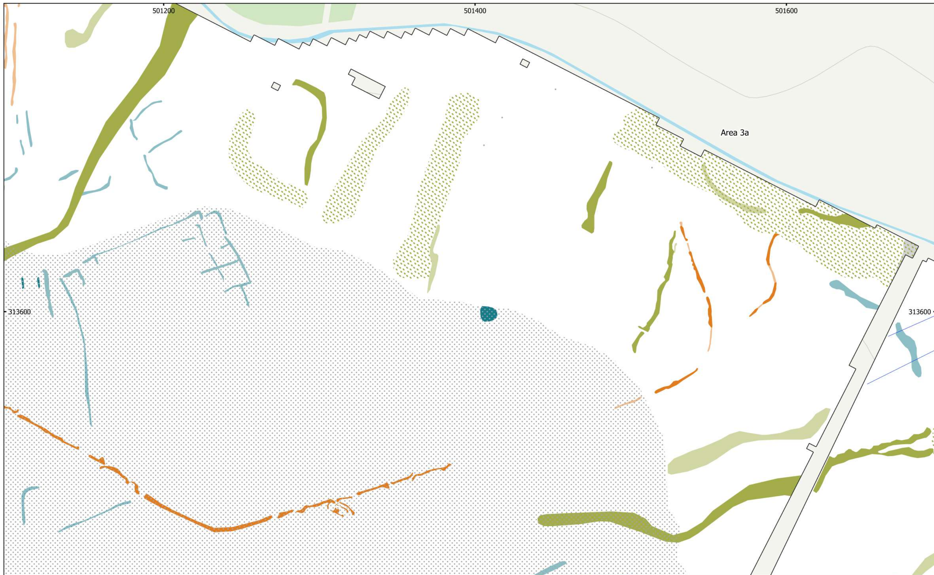
MSTF1136: Mallard Pass, DCO, Essendine, Rutland Figure 28 - Magnetic Interpretation (Area 3a) 1:1,500 @ A3 Copyright Magnitude Surveys Ltd 2022 Contains Ordnance Survey data © Crown Copyright and database right 2022
