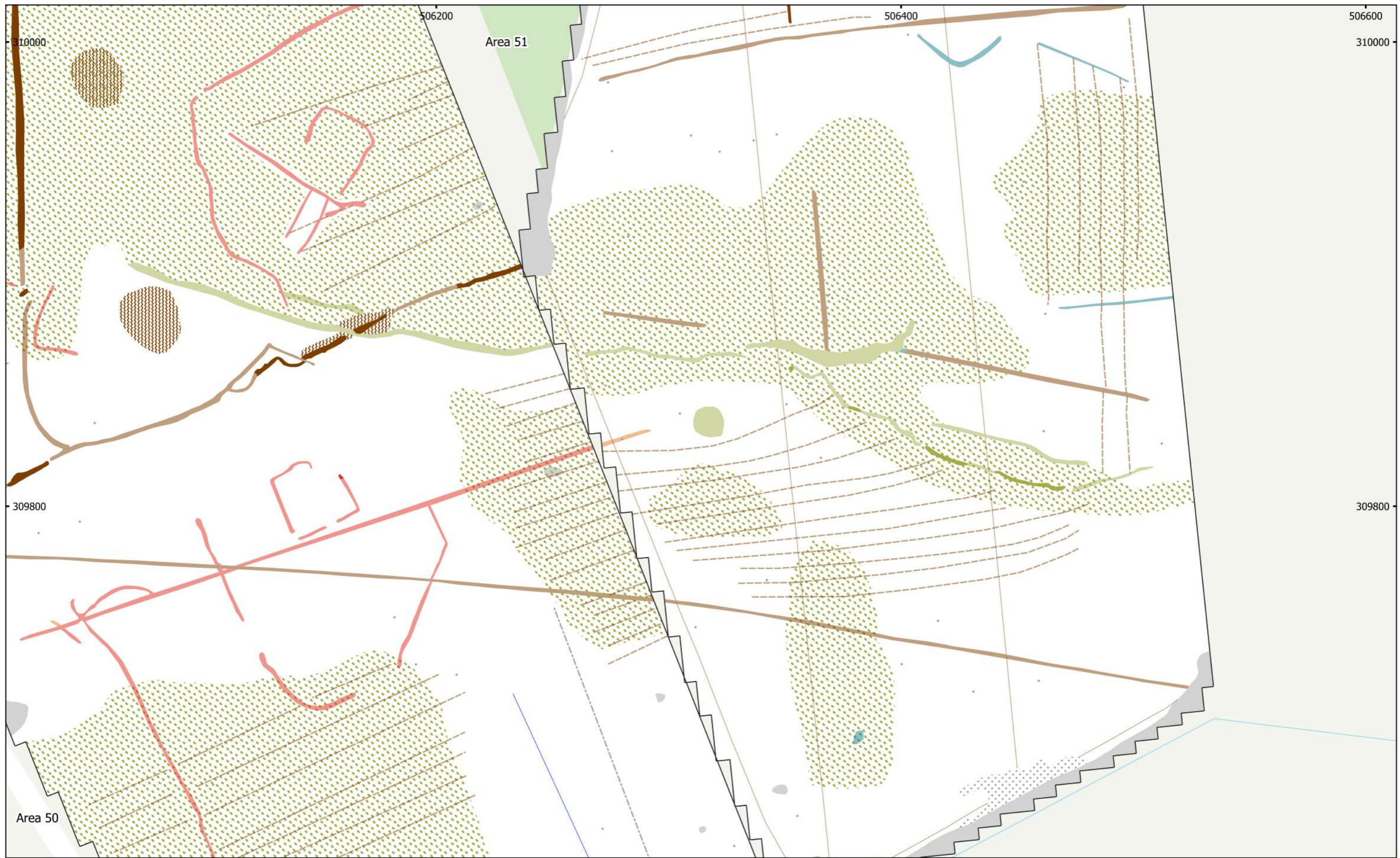
MSTF1136: Mallard Pass, DCO, Essendine, Rutland Figure 172 - Magnetic Interpretation (Area 50 & 51 (South)) 1:1,500 @ A3 Copyright Magnitude Surveys Ltd 2022 Contains Ordnance Survey data © Crown Copyright and database right 2022
