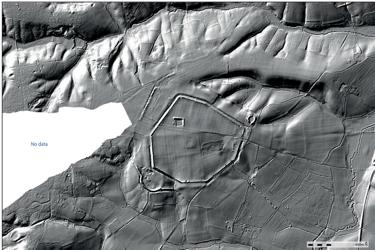
FIG. 3.14 The Environment Agency LiDAR data around Silchester, supplied by their Geomatics Group. The data show a composite of surveys (created November 2012) predominantly at 1 m resolution.
