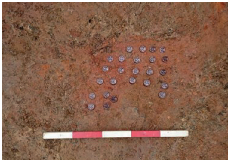
FIG. 136. Archaeomagnetic sampling of LL3 (Context 1139). Specimens numbered 1 to 25 consecutively, from left to right, starting at the top of the image. Specimen number 25 sits between specimens numbered 22 and 24. Image taken facing north-west, 0.50 m scale (Photo: Harris 2017)
