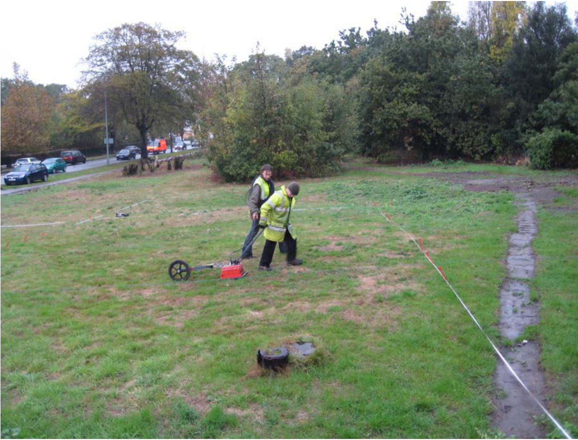
Fig 8 Ground penetrating radar (GPR) survey in progress due south of the position of backfilled evaluation Trench 1 at the S end of the site (looking N)
