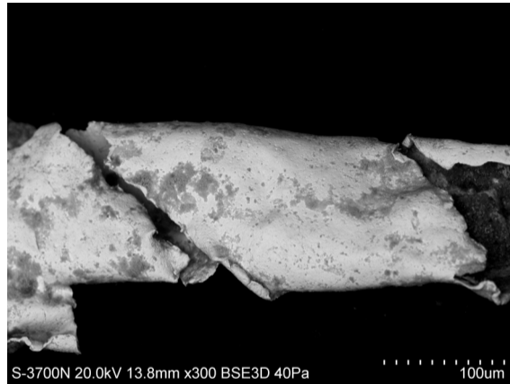
Data Fig 39 SEM images of gold thread fragments <191>b (left) and <191>f (right); note natural curling of strip along edge (images A Mongiatti) (W of view c 0.25mm (left), c 0.4mm (right))
