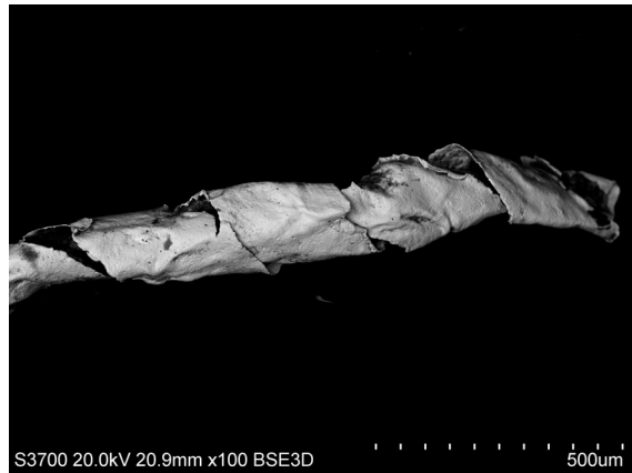
Data Fig 35 SEM images of gold thread fragments <191>a (left) and <191>e (right), showing thinness of strip, tight spinning of thread and overlapping of gold strip, damage on strip and flattened areas (lower end of fragment <191>a, left) (images A Mongiatti) (W of view c 4mm (left), c 1.5mm (right))
