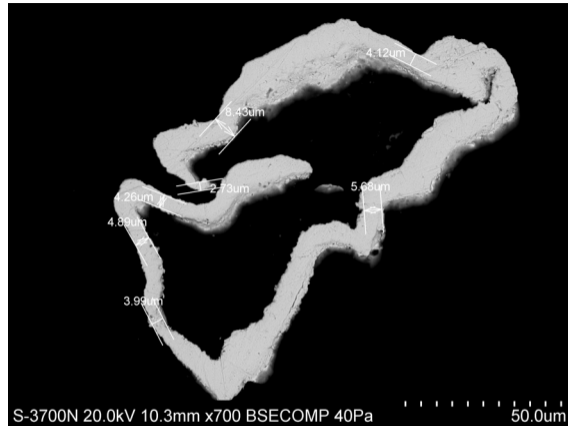
Data Fig 44 SEM images of further polished cross-sections of gold thread fragments <191>b (images A Mongiatti) (W of view c 80 μm (left), c 175 μm (right))
