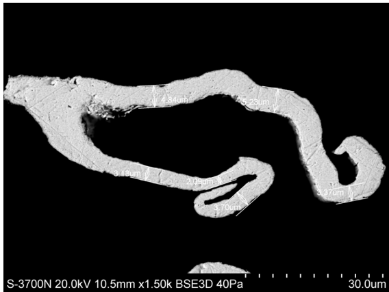
Data Fig 42 SEM images of polished cross-sections of gold thread fragments <191>b, showing how edges of strip have curled and are thinner than core (images A Mongiatti) (W of view c 80 \mu m (left), c 100 \mu m (right))
