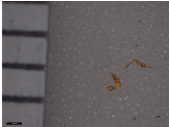
Data Fig 34 Spun gold thread fragment <191>b cut in half (left) and one half of <191>b further cut in half with fine scissors (right) (photos A Mongiatti) (scale graduation 1mm)
