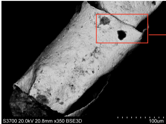
Data Fig 40 SEM images of gold thread fragment <191>e showing cutting-tool marks on edge of gold producing very thin edge (images A Mongiatti) (W of view c 0.35mm (left), c 0.1mm (right))
