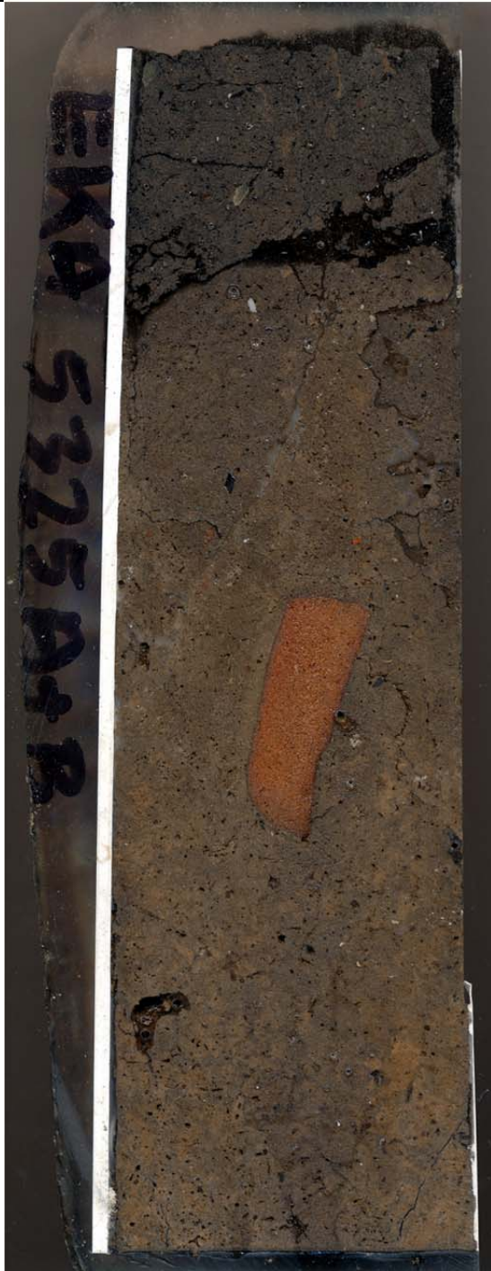
Fig. 18: Scan of resin embedded block M5325A&B, showing humic Roman dark earth topsoil formed in brown earth, with anomalous irregular boundary between the upper more humic (2.39% LOI) topsoil and less humic subsoils (1.61% and 1.29% LOI, respectively). Note large pot fragment, also present in thin section M5325B. Height is ~18cm.
