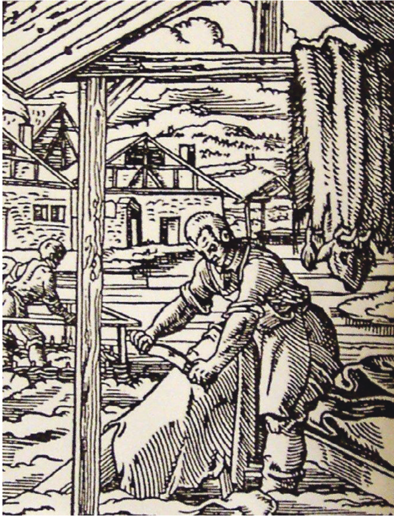
Figure 39: German woodcut of 1568 of a tanner at work, showing a cow hide hanging up with the horns and tail still attached (after Serjeantson 1989)
