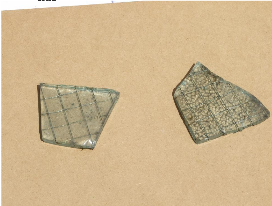
Figure 31 - Fragments of reinforced glass found beside the turning circle the western end of the hospital tramway (glass designed by Pilkingtons in 1898)
