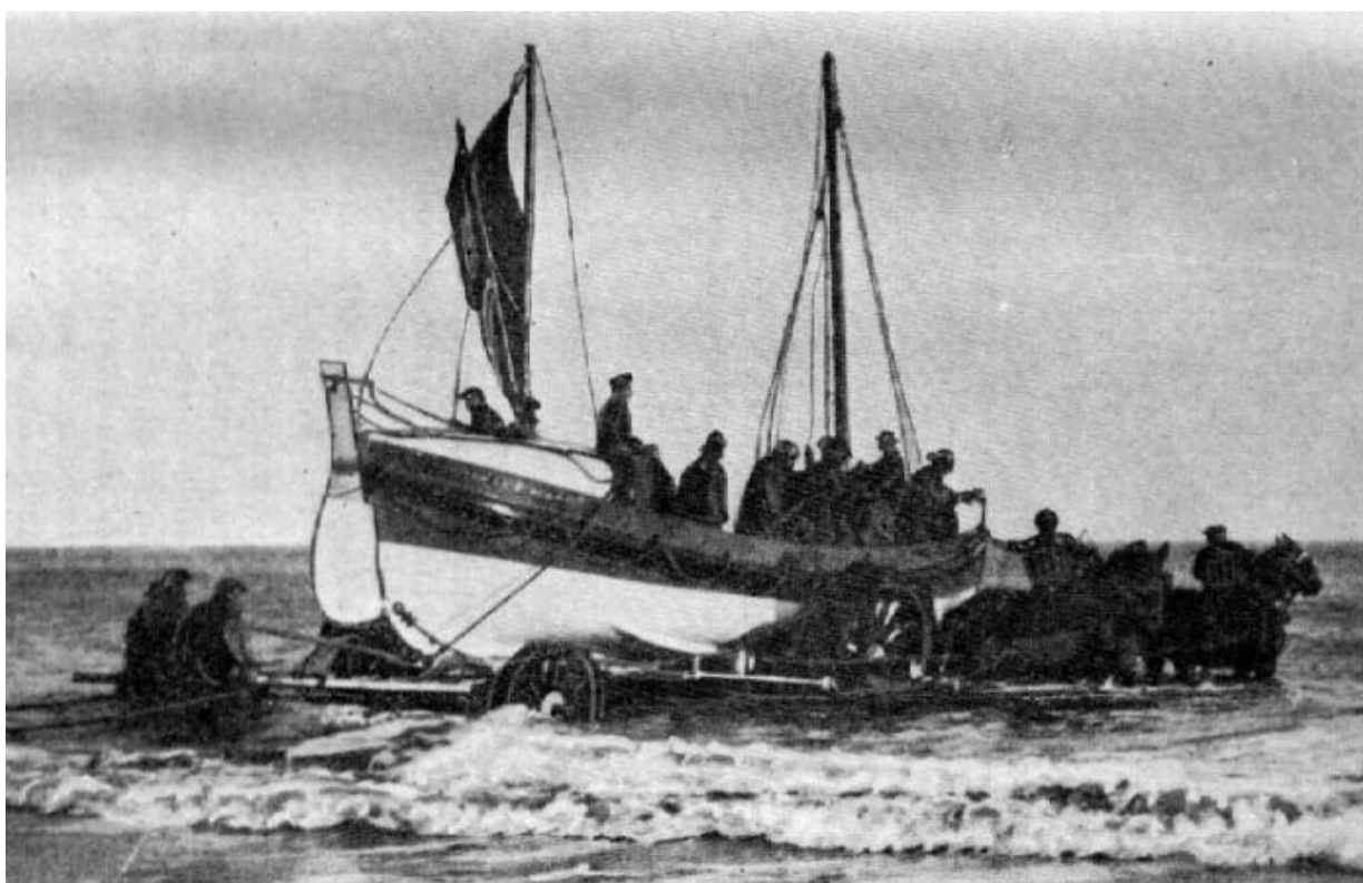
Launching the Bridlington Lifeboat in more clement weather. This shows how the horses were hitched either side of the carriage, rather than directly in front of it. Also visible are the large sand-plated wheels, one of which was shattered when the Lifeboat was swept off the carriage.
