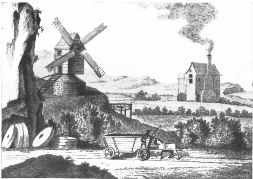
Propelling a rail vehicle by horse in County Durham. This unusual view, showing a railway coal wagon with horse in rear, is reproduced from the illustrated title to the map of the County Palatine of Durham, surveyed by Captain Armstrong and engraved by Thomas Jeffreys, 1768. It is suggested that the apparent "shaft" is a brake lever.
