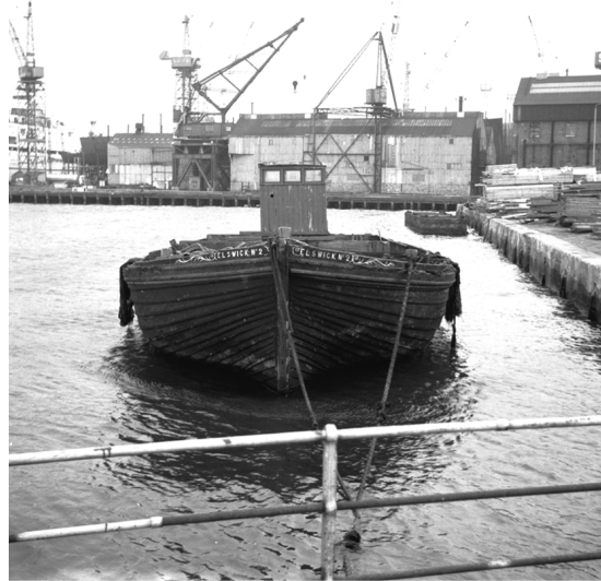
Fig. 15 Elswick No 2 at Tyne Dock, as donated to Tyne and Wear Museums in 1976. By this time she had been fitted with a diesel motor and a small wheelhouse aft. (Copyright Beamish Museum. Reproduced by kind permission of Beamish Museum. Photo No: 3746).
