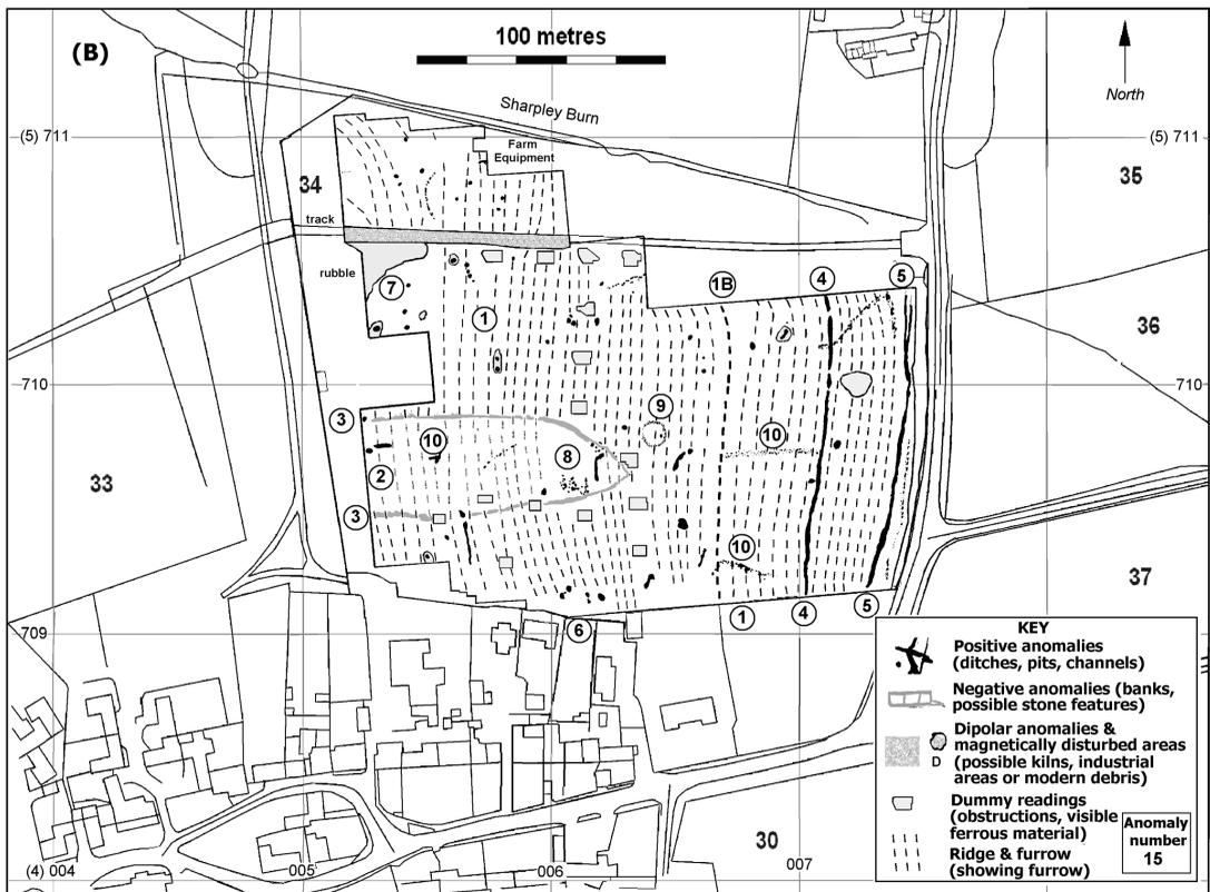
Fig. 11B Annotated anomaly plan for magnetic survey of Field 34. Map made using OS/EDINA cartographic data, © Crown Copyright.
