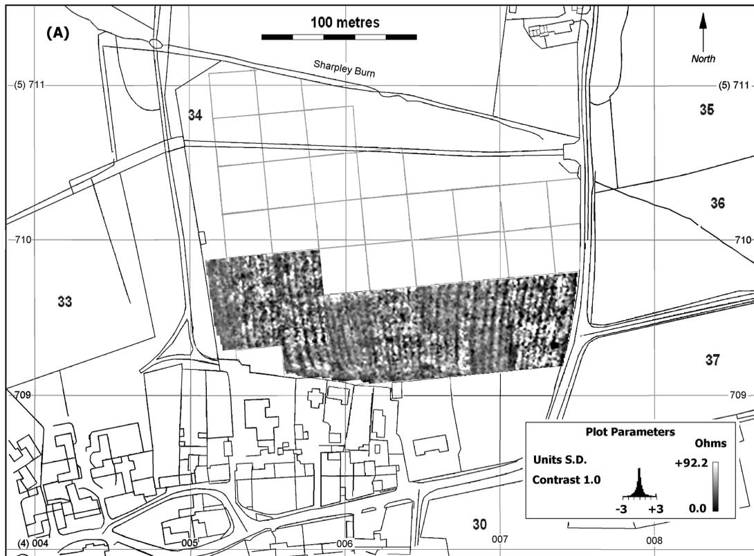
Fig. 12A The resistivity survey of Field 34. Map made using OS/EDINA cartographic data, © Crown Copyright.
