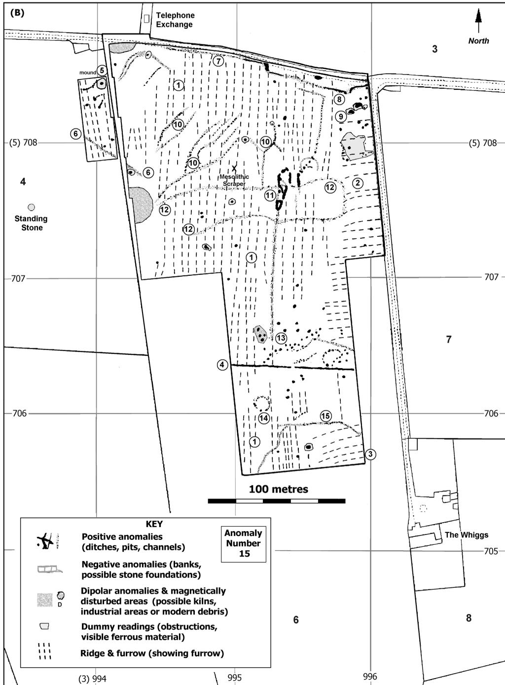
Fig. 14B Annotated anomaly plan for magnetic survey of Field 6. Map made using OS/EDINA cartographic data, © Crown Copyright.
