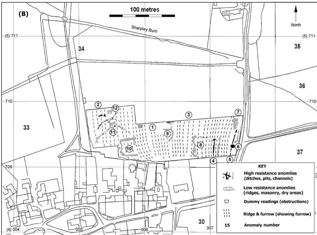
Fig. 12B Annotated anomaly plan for resistivity survey of Field 34. Map made using OS/EDINA cartographic data, © Crown Copyright.
