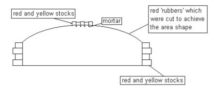
It was tentatively suggested that the vaulting had been constructed using a wooden framework as a guide and support during construction from above - this was proposed to explain why mortar postholes beyond the brickwork. It is possible that the mortar dump 166 found immediately above the floor 191 relates to the construction of the ceiling or to the construction of the blocking walls. (Plan 166)
