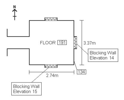
Blocking wall 188 was comprised of red and yellow stocks laid on bed in alternate rows of headers and footers (resembling English Bond) which have been bonded onto 134. It was faced on both skins and was rubble infilled.
