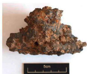
Figure 3. Fragment of dense iron silicate
