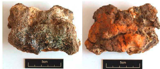
Figure 2. Vitrified ceramic, probably the remains of smithing hearth or smelting furnace (inner surface = left, outer surface = right)
