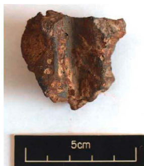
Figure 4. Fragment of dense iron silicate showing abundant charcoal impressions
