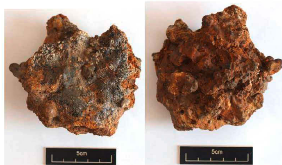
Figure 1. Smithing slag cake (upper surface = left, lower surface = right)
