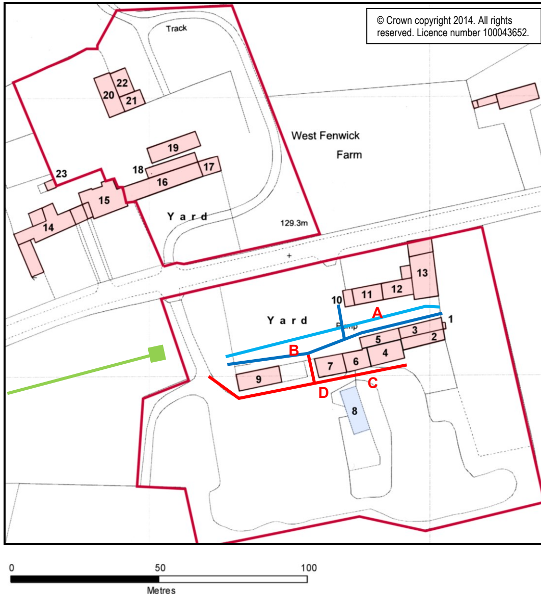
Figure 2: The building ranges of West Fenwick Farm. Building 8, in blue, has been partially demolished. North is to top of page. Excavations monitored (in green, red and blue) are described in section 6. Red letters (A, B, C and D) indicate location of illustrated sections.
