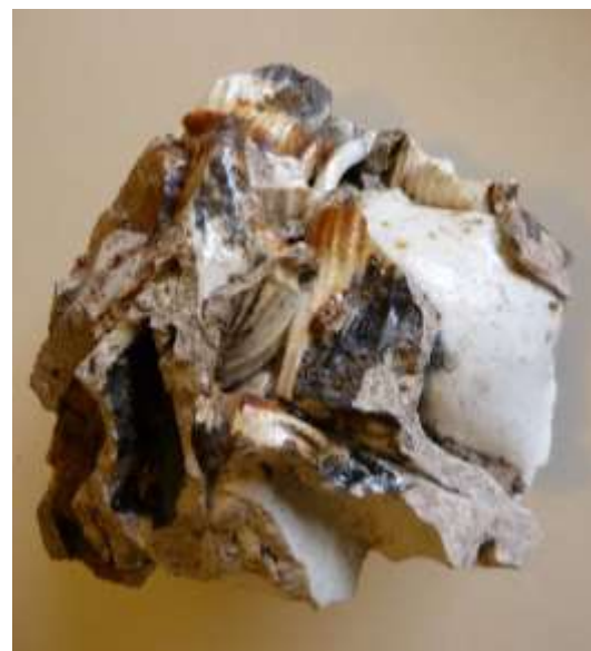
Plate 10: Overheating of a kiln during a glaze firing melted a batch of ribbed marmalade-pots in a saggar. Stilts, for separating the pots during the firing, can be seen attached to the saggar wall in the left hand photograph. Recovered from infill of the clay pit.
