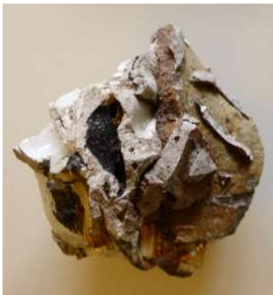
Plate 10: Overheating of a kiln during a glaze firing melted a batch of ribbed marmalade-pots in a saggar. Stilts, for separating the pots during the firing, can be seen attached to the saggar wall in the left hand photograph. Recovered from infill of the clay pit.
