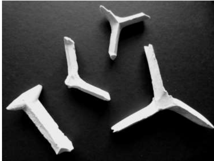
Plate 9: Kiln furniture from dumped deposits within the clay pit. To right is a stilt, the remaining three are 'cockspurs' all fragmentary. All were for stacking pots during a glaze firing.
