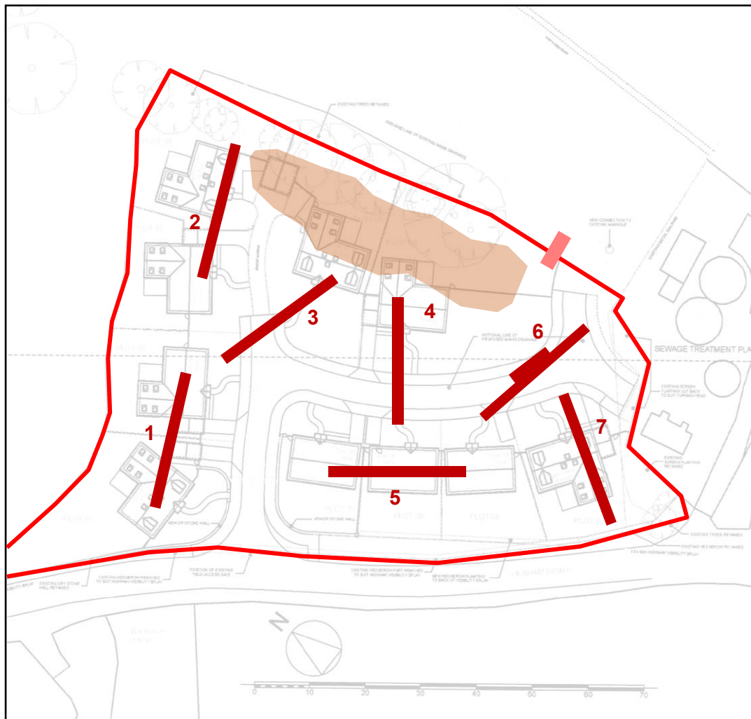
Figure 3: proposed development plan (grey background) of the PDA with evaluation trench locations (1 to 7) in red. All trenches are 25m long by 1.6m wide. Area in pink tone shows modern trackway cut through bank. Brown tone shows modern spoil heap from developments on Mote Hill.
