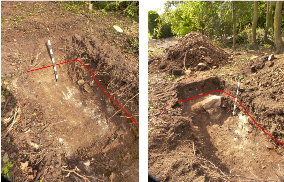
Plates 11 and 12: Test pits 1 and 2 in the footprint of the ramp between forecourt and western drive. Red line indicates surface of sandstone bedrock 1m scale.
