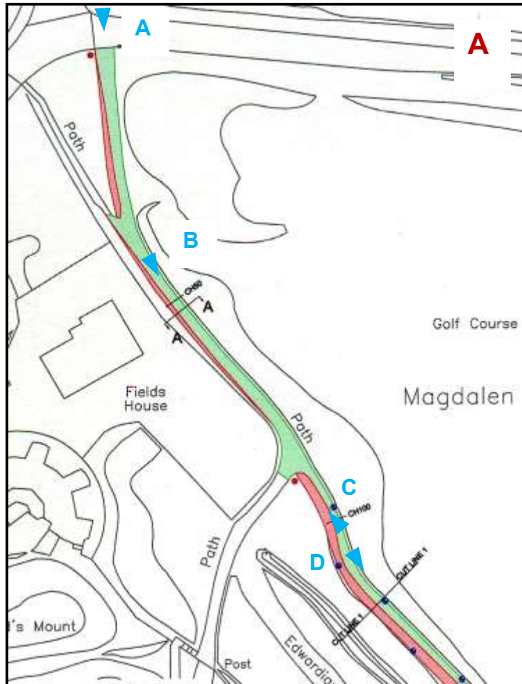
Figure 5: Northern area of footpath works (see figure 4). Green tone: existing path; Pink tone: path to be widened; red dot: finger post; blue dots: LED demarcation lights. Blue arrows locate plates A to D. From NCC drawing HE141308- 16/00U107/01/01.
