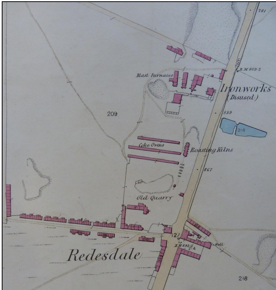
Figure 14: First Edition Twenty Five Inches to One Mile Ordnance Survey of Ridsdale (1860). The ironworks is dormant. At the time, Forster was negotiating for funds to re-open the site prior to his premature death the same year. The map shows all the structural components of the works and specifically names the blast furnaces, ore roasting kilns and coke ovens. Also shown are waste heaps and quarries. A reservoir lies to the east of the A68. This supplied water to boilers of steam engines located immediately to the south of the engine house.
