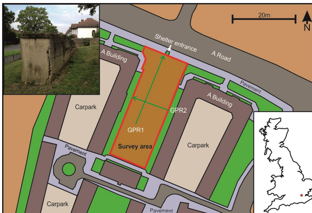
540 541 Figure 17. South London study site 3 map (location map inset), showing the 542 geophysical survey area, the entrance (photograph inset) and the two GPR 2D profile 543 locations shown in the paper. Map courtesy of EDINA™ DigiMap (2016).
