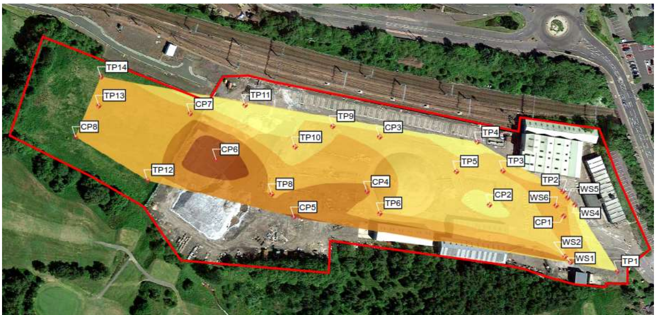
Plate 3 – GIS Plot highlighting the distribution of made ground (see Figure 2 for detail), the darker colours indicate deeper deposits.
