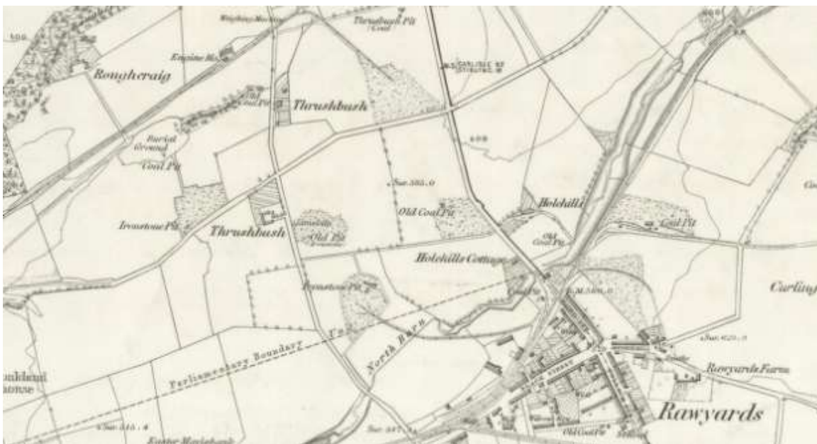
Plate 3 – Excerpt from 1 st Edition Ordnance Survey Six Inch, 1859, Lanarkshire, Sheet VIII (includes: Bothwell; New Monkland; Old Monkland; Shotts) highlighting the early growth of industrial activity spreading out from Rawyards towards the Site. This can also be seen with the appearance of coal mines and a rail network in the area. Reproduced with permission of the Trustees of the National Library of Scotland.
