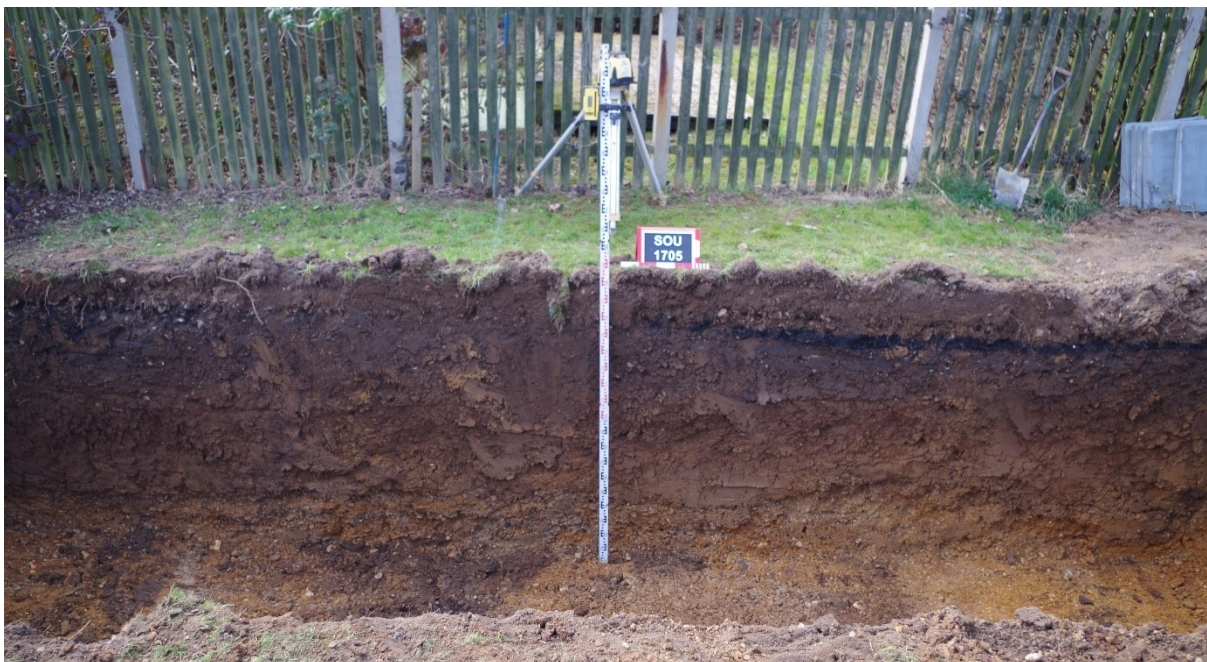
Figure 6. Section showing natural gravel and brickearth deposits in the southeast of the site in soakaway trench 20. Trench is 1.8m deep.
