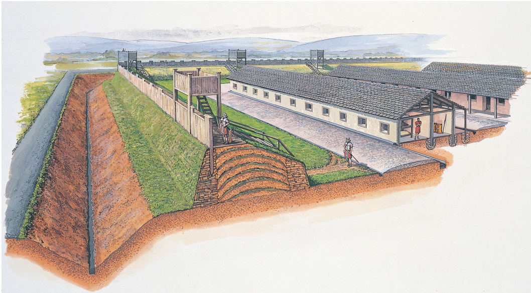
Fig. 7a. Reconstruction drawings of the Phase I earth and turf rampart. Note that there is no evidence for the timber turrets shown in the Phase I reconstruction.
