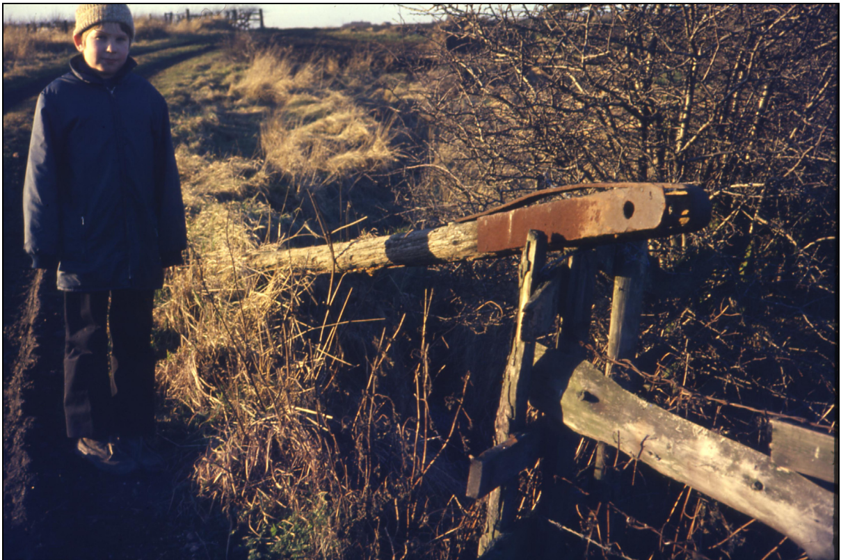
Plate 17: photograph by Don Wilcox showing pump spears from Crowtrees Colliery used as a fence rail (not found during 2009 survey). These timber spears were joined together to form a linkage to transfer power from the steam engine to a pump at the bottom of the shaft (c. Durham District Council).
