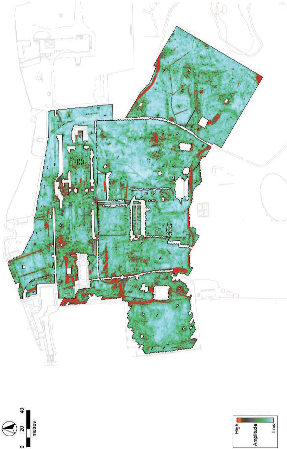
Fig 2.11 GPR data (migrated and filtered): timeslice 0.0m-0.5m (© Claire Stephens, GSB Prospection)
