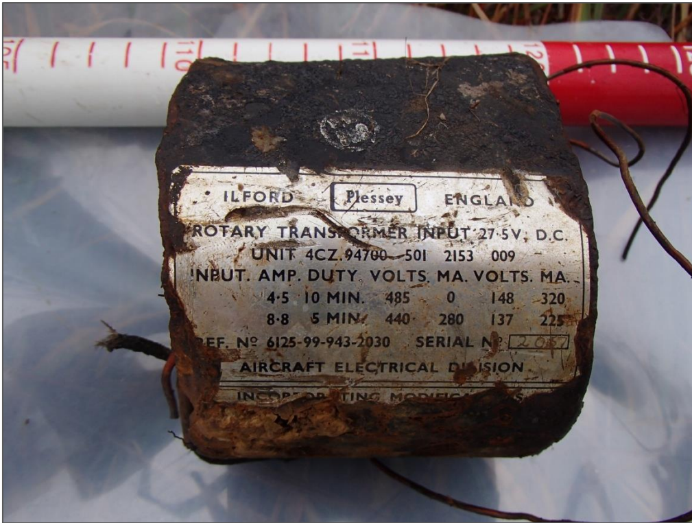
Plate 39 1764.32 Close up of rotary transformer.
