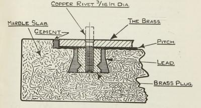
4.—Place the brass temporarily in place. Mark off the rivet holes, drill and tap for the rivets.
