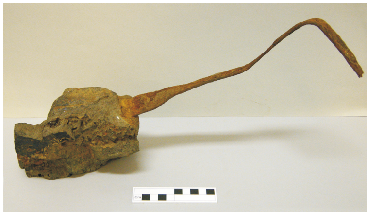
Fig 12 Cast slag block with iron strip from Coxes Lock, Addlestone. (Photograph by kind permission of Chertsey Museum, ref CHYMS-3237)
