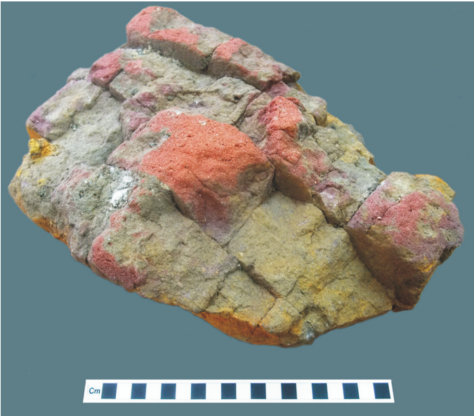
Fig 9 Lower surface of flowed slag, with small quartz-rich bricks
