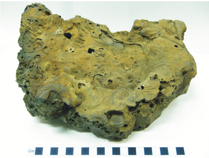
Fig 10 Downside Mill, Cobham. Large slag mass from the tail-race lining.
