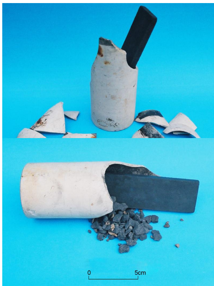
Figs 18 (above) and 19 (below) Cylindrical vessel of unglazed stoneware containing a mixture of mined graphite and a manganese ore together with a graphite bar
