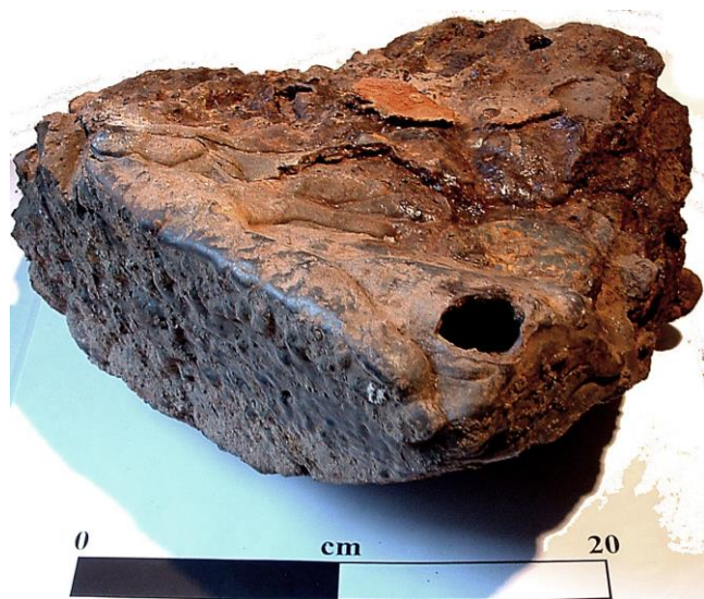
Plate 2. Fayalitic block from context 020. Probably the best indication of a finery or similar process for converting pig iron to wrought iron
