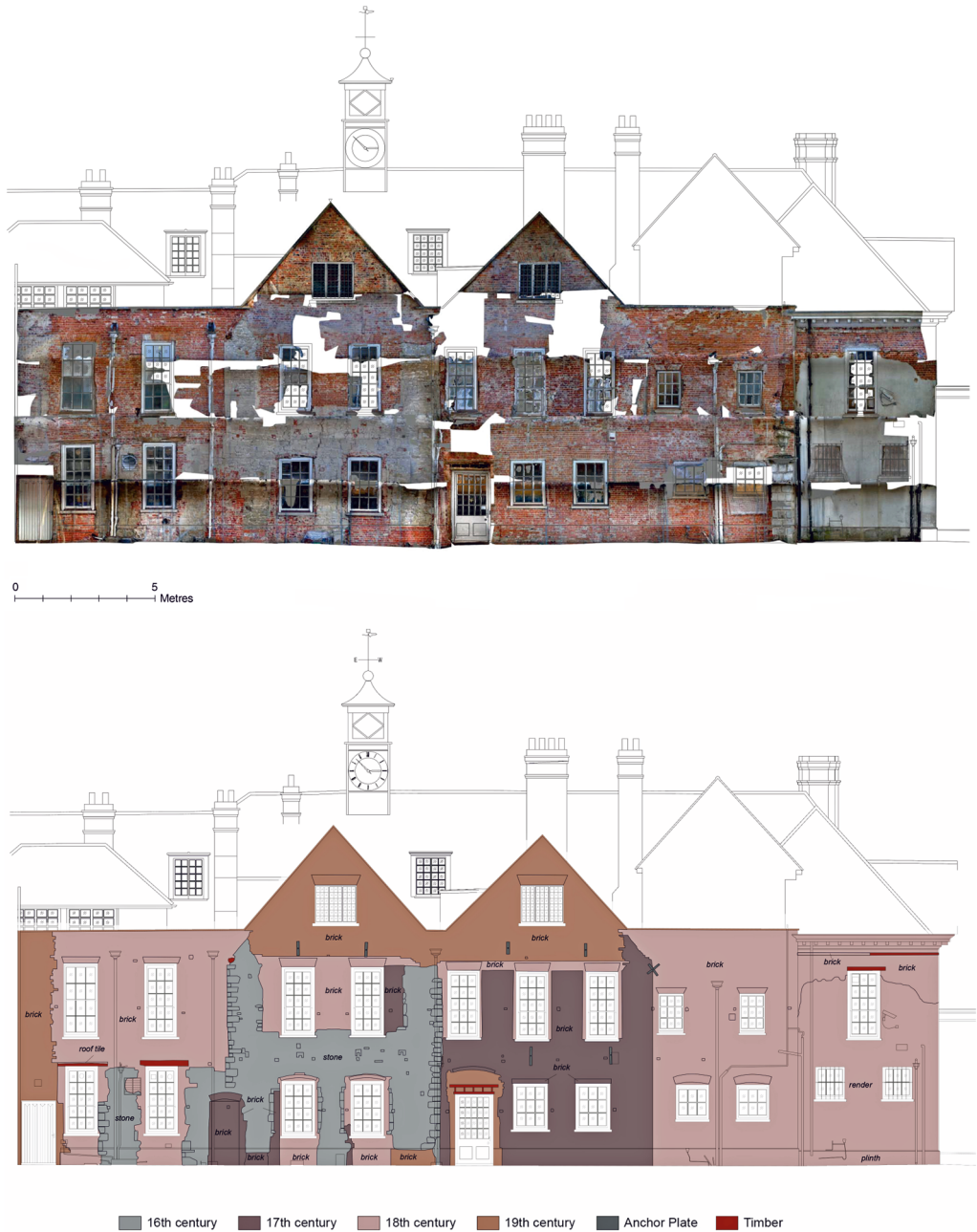
Fig 1 Reigate Priory Junior School, Bell Street, Reigate. (top) A rectified photographic survey shows the north-facing elevation of the principal building of the open courtyard, following the removal of much of the later render, revealing the different fabrics used in its construction; (above) An interpretation of the date of construction of the various elements of the building based on fabric type. (© Lewis Brown Chartered Land Surveyors)
