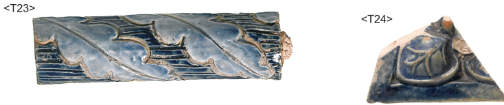
Fig 23 Doulton Terra Cotta Works. Faience; glazed terracotta column from a window arch (<T 23>) and panel with palmette decoration (<T 24>) (scale 1:4).
