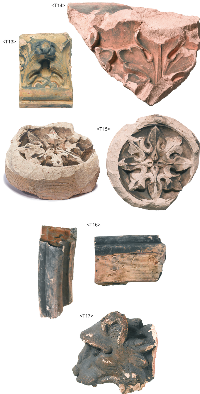
Fig 19 Doulton Terra Cotta Works. Terracotta mouldings; string courses (<T 13>–<T 14>), medallion (<T 15>), window moulding (<T 16>) and probable winged grotesque (<T 17>) (scale 1:8, except <T 14> and <T 17> scale 1:4).
