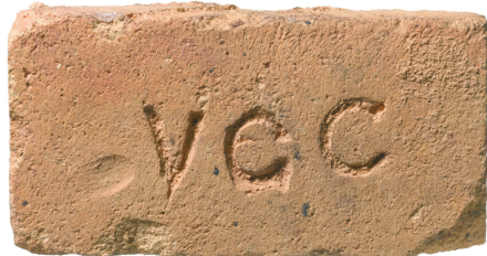
Fig 16 Doulton Terra Cotta Works. Stamped firebricks used in the Doulton kilns and flues; Cowen (<T 1>), Stephenson (<T 2>), Starworks Glenboig (<T 3>) and VGC (<T 4>) (scale 1:4).
