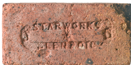
Fig 16 Doulton Terra Cotta Works. Stamped firebricks used in the Doulton kilns and flues; Cowen (<T 1>), Stephenson (<T 2>), Starworks Glenboig (<T 3>) and VGC (<T 4>) (scale 1:4).
