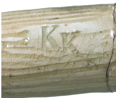
Fig 27 Doulton Terra Cotta Works. Examples of stamped lettering 'NN' and 'KK' on the backs of faience pieces (<T 28> and <T 29>) (scale 1:1).
