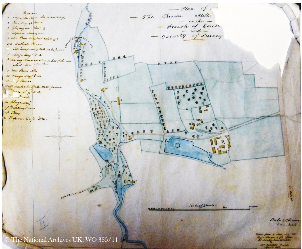
Fig 2 Ewell Gunpowder Mill. Plan of 1863 when the mills were in the ownership of Sharpe & Co. The Incorporating Mills are the most northerly of the eighteen structures or groups of structures noted on the plan as comprising the mill complex. The structures were spread out to minimise any explosion damage.
