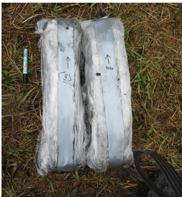
Fig. 5.11. Monolith samples wrapped and ready to be taken for laboratory analysis.
