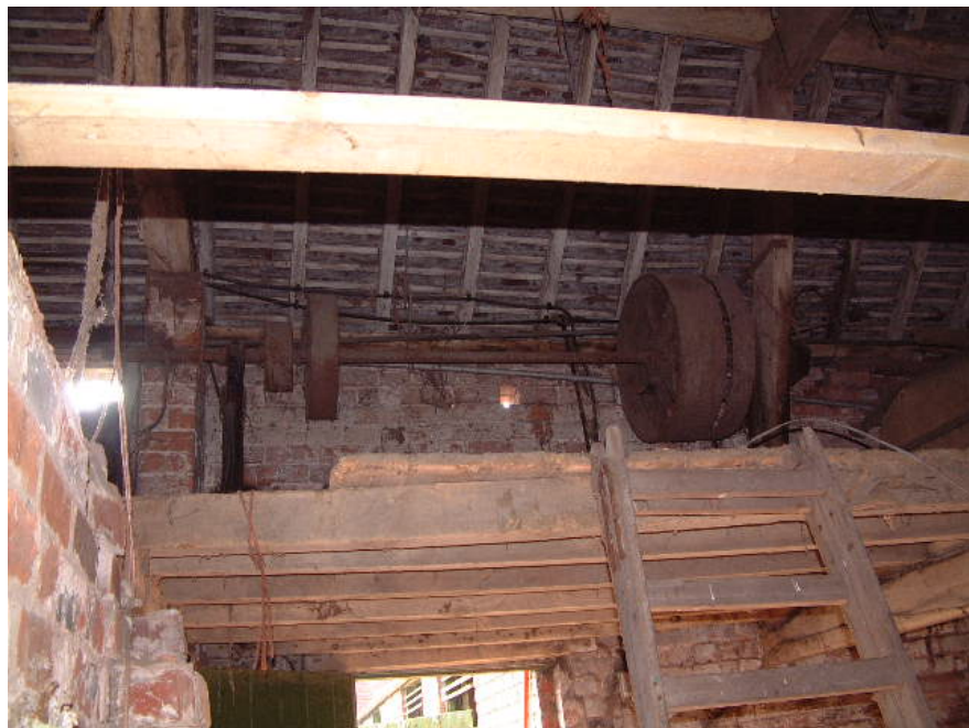
Flywheels and shaft for 19 th century machinery power train in Building 2
