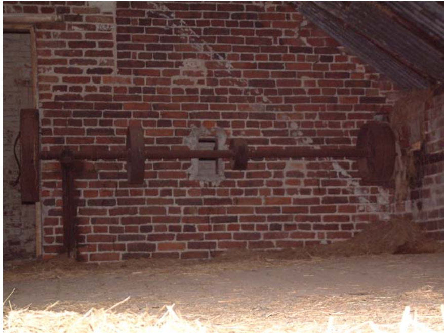
Belt wheels and shaft inside the fodder processing shop, note the former eaves height of the building as a mark on the wall
