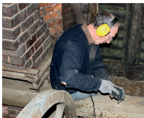
Fig 3 Tree-ring dating being carried out on the late 17th-century bellframe at Kirklington St Swithin (Photo: CJ Brooke)
