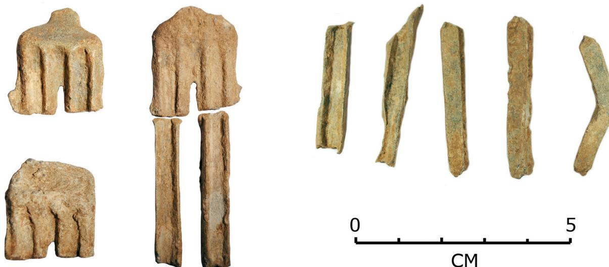
Fig 3 Thornton Abbey, Lincolnshire, casting waste and off-cuts from lead came manufacture (Image: H. Willmott)
